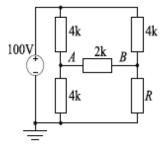
14. [D] Calculate  $V_X$  in the following circuit. You can either use nodal analysis directly or else simplify the circuit a little to reduce the number of nodes.
